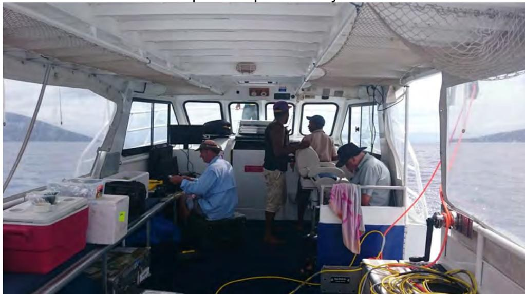
Fig 1 – MV Karavas with cantilevered pulley system for orange spectra shot line attached to the flying clump and ROV yellow umbilical in Starboard waist opening.
